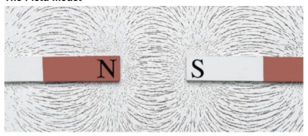
The photo shows the patterns of iron filings formed when they are around a magnet.
