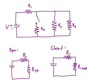
What happens to the voltage across each resistor when the switch is closed?
